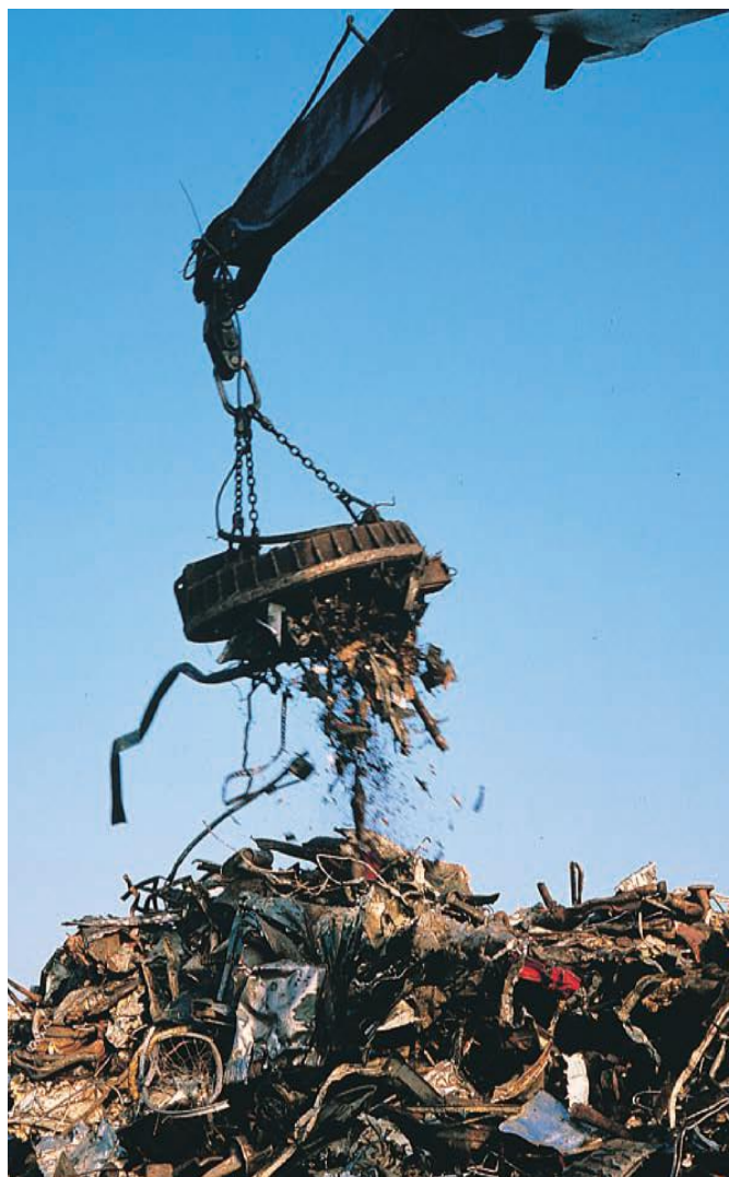
Figure 45.7 Electromagnet being used to lift scrap metal
